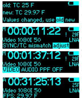
If settings are changed, confirmation is required: Pushing the config switch while "old" is highlighted, discards the changes and returns to the main menu. Pushing the config switch while "new" is highlighted will set the time code signal to the selected rate. If the selected time code frame rate is incompatible to the currently set video signal type, a warning message appears:
