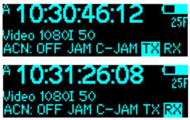
**TX** is a wireless transmission of external time code present on the Lemo/TC input. This is intended for transmitting a record-run time code to another ACN-TL or ACL 204 which is in **RX** mode.
