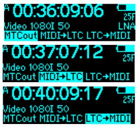
MTCout: this is the default mode. The ACL 204 always puts out MTC, unless the USB port is set to COM (see SYS > Config > USB).
