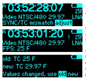
You have no choice but to press the config switch and are automatically taken to the time code rate setting:
